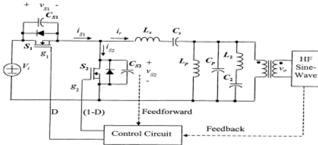
Fig.2 Proposed APWM resonant inverter topology
