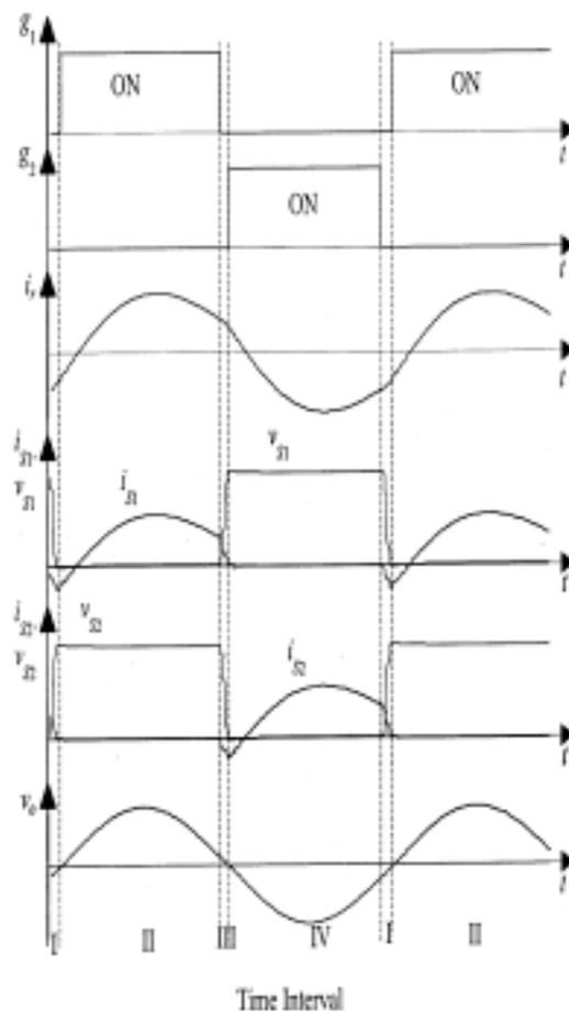
Fig.3 operating waveforms of the inverter.
