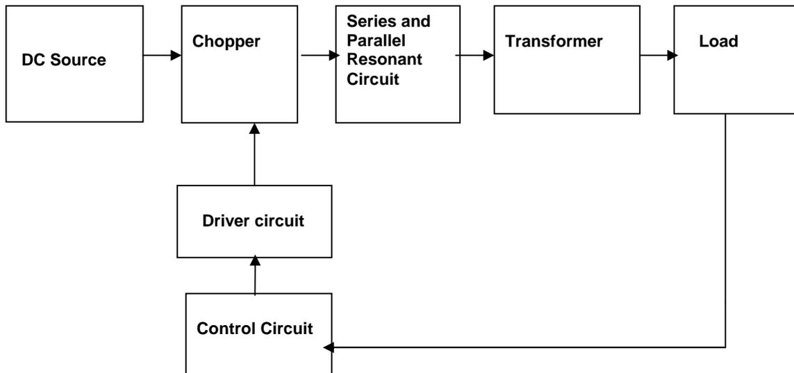
Fig.1. Block diagram of Proposed APWM resonant inverter topology
